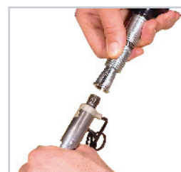
Rotate anticlockwise and release the tool ring
